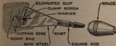
A Tool Made from a Few Scraps of Steel is Useful for Fitting Instruments to the Dashboard
